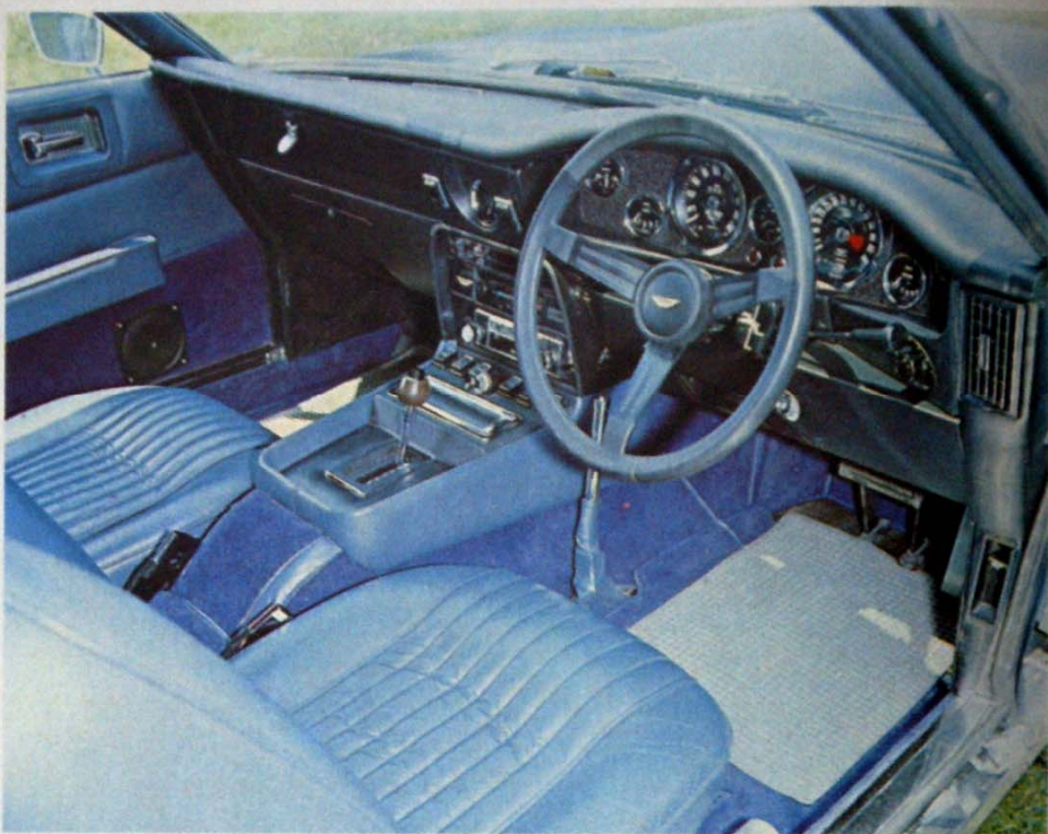
Embossed leather upholstery, a full complement of instruments, and sensible sighting of the controls all add up to the finest in Grand Touring comfort. Power steering permits the use of a small diameter steering wheel, while the selector lever for the Chrysler Torqueflite automatic gearbox falls readily to hand
