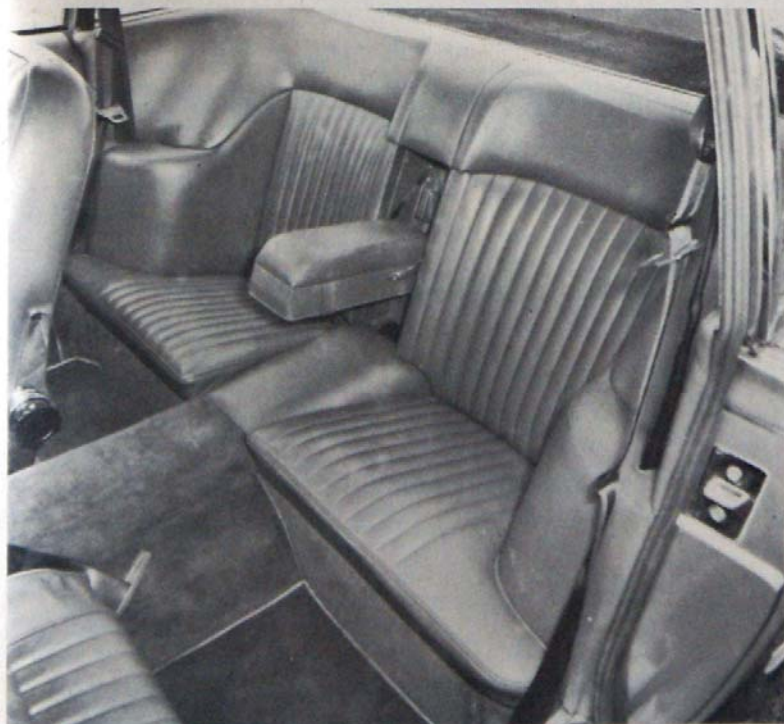
Left: at the rear, the seats are well shaped, with small armrests at the outboard ends; note the very neat fitting of the seat belt to the transmission tunnel
