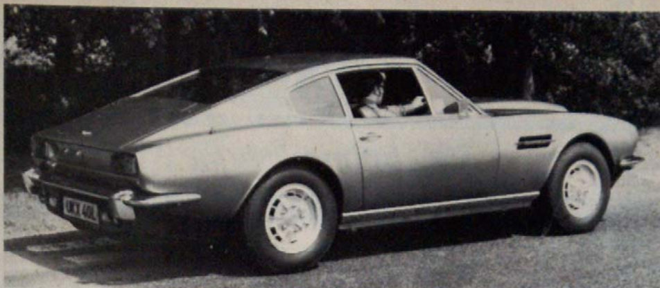
The dual fuel filler caps, below the rear screen, are no longer fitted with locks; light alloy wheels are standard
