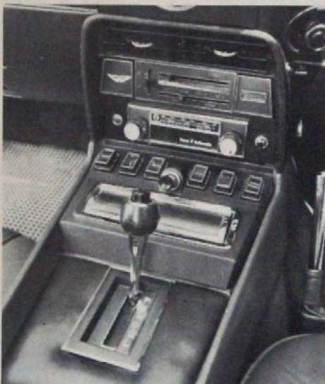
Above: Push-button switches replace the previous rocker types, and the air-conditioning panel has been completely redesigned
